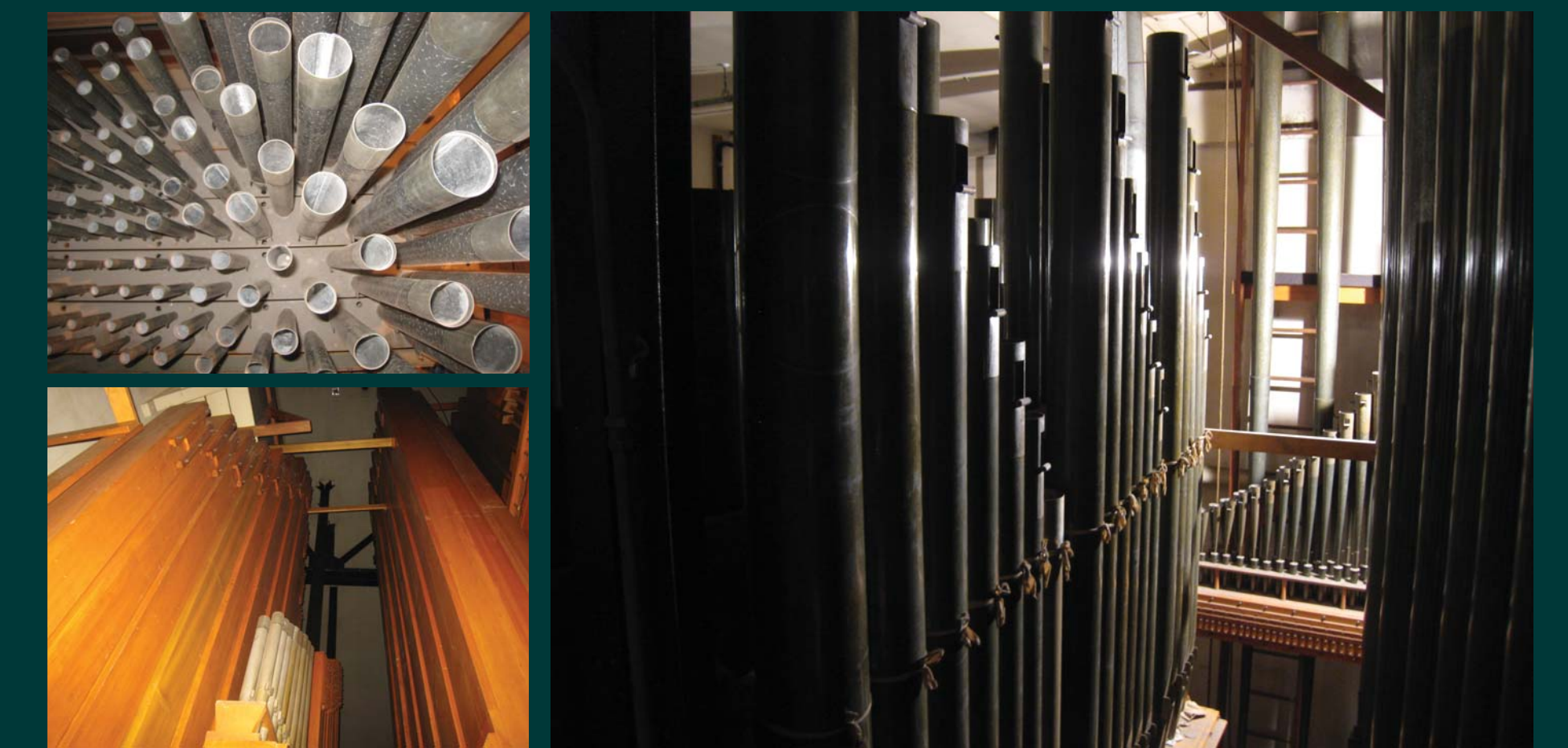
Figures 4-6: The organ's nearly 7,000 pipes are located in a series of six rooms in the Northrop Attic. There are four ranks and 108 stops. The pipes were all handcrafted by the Aeolian-Skinner Organ Company and installed in four sections between 1932 and 1935.
