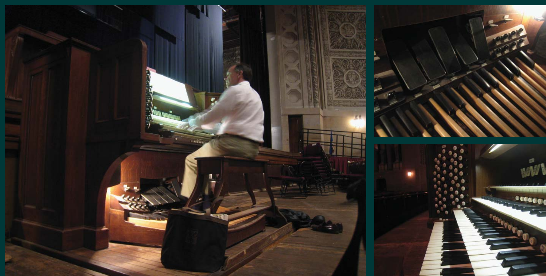
Figures 1-3: The Organ Console, located on the main floor in the orchestra pit. It connects to the pipes through a series of cables that run through the walls. The console is set on a hydraulic lift so it can lower into the floor.
