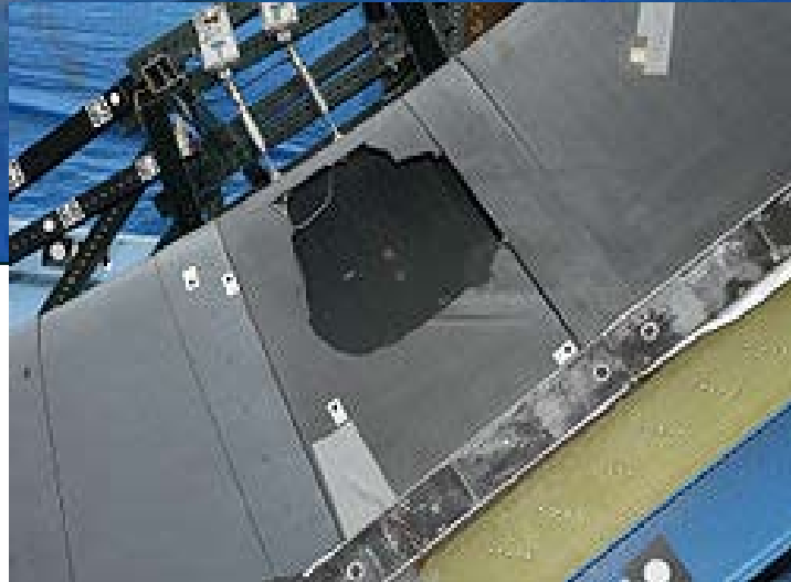
Simulated test results reveal fuel pod foam damaged Columbia's left wing at lift-off
